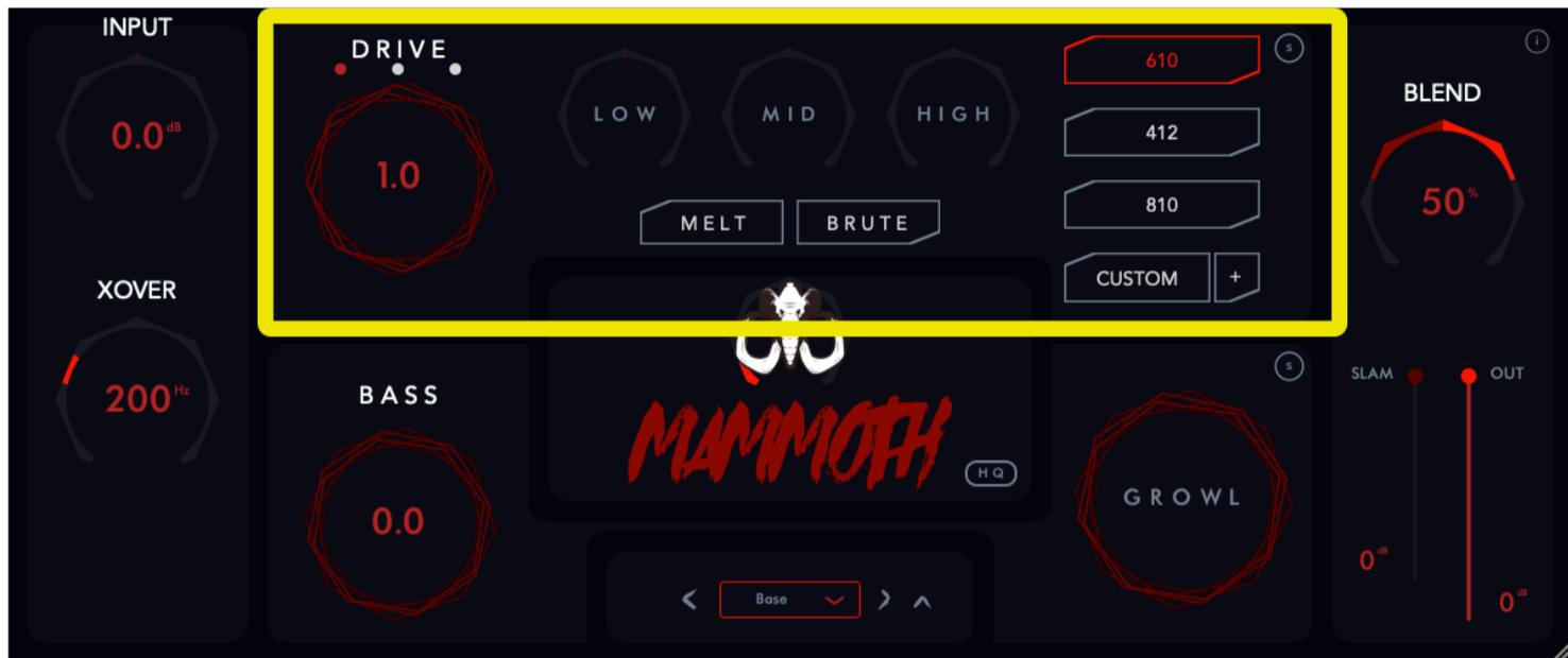
After the crossover, within the HIGH section, the signal is processed by a preamp model and an IR loader (convolution). You can choose between 3 totally different modeled circuits:
